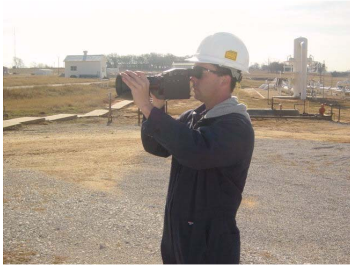
IR camera in use for DI&M - Source: Leak Surveys, Inc.
