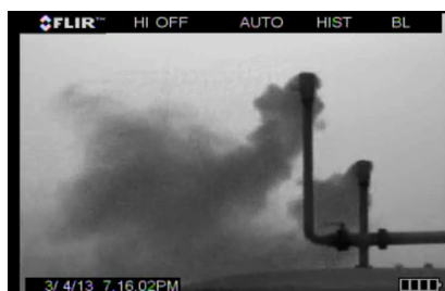
SHALE TEST INFRARED VIDEO: Recorded VOC Emissions FLIR GasFindIR Camera
