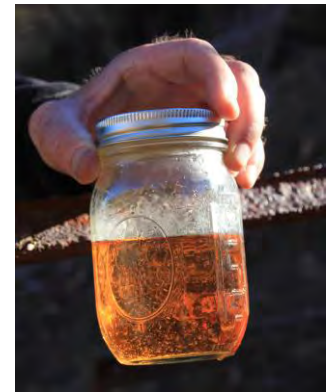
Acid mine drainage and metals leaching could permanently contaminate groundwater. This sample, heavy in iron and other metals, is highly acidic and was collected from a small Arizona mine.
