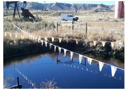
Skim pits are used to separate oil from produced water and are death traps for wildlife. Flagging is an ineffective deterrent for preventing wildlife mortality in oil pits. Photo by Pedro Ramirez, Jr./USFWS
