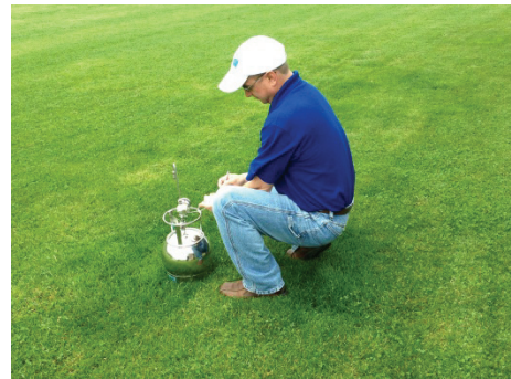
Placing an air canister at a test site for collecting emissions data.
