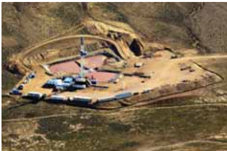
FIGURE I-36. CONVENTIONAL DRILLING SITE This site, with reserve pits disturbs 3-4 acres of land. Photo by Jonathan Selkowitz
