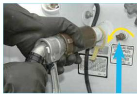
If necessary, open the vent on the fixed maximum liquid level gauge.
