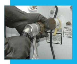
Slowly loosen the nozzle to vent any propane liquid trapped between the nozzle and the fill valve or remote fill connection. Wait until propane stops venting and pressure is relieved between the nozzle and the fill valve before completely disconnecting the nozzle. If propane does not stop venting, retighten the nozzle and contact your supervisor. When venting stops, disconnect and stow the hose assembly.
