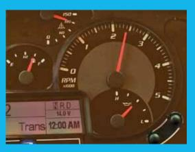
For most driving conditions, engine speeds between 2000 and 2500 rpm achieve the best fuel economy. Listen to your engine to get a feel for fuel-saving starts and gear changes.
