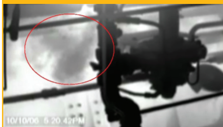
Figure 36: Leaking Valve as shown by Infrared Gas Detector
