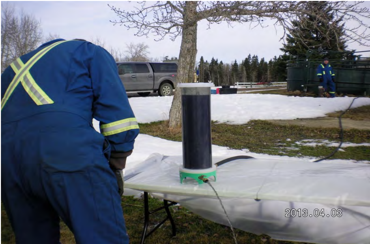
The Campbells' contaminated well water being gas tested in a flow-through cell for the ERCB, April 3, 2013 The black in the cell is the Campbell's water; it took 20 minutes to clear. The well is plastic lined and had not been used for about a year. (Flow-through cells are about 15% efficient. 373 )
