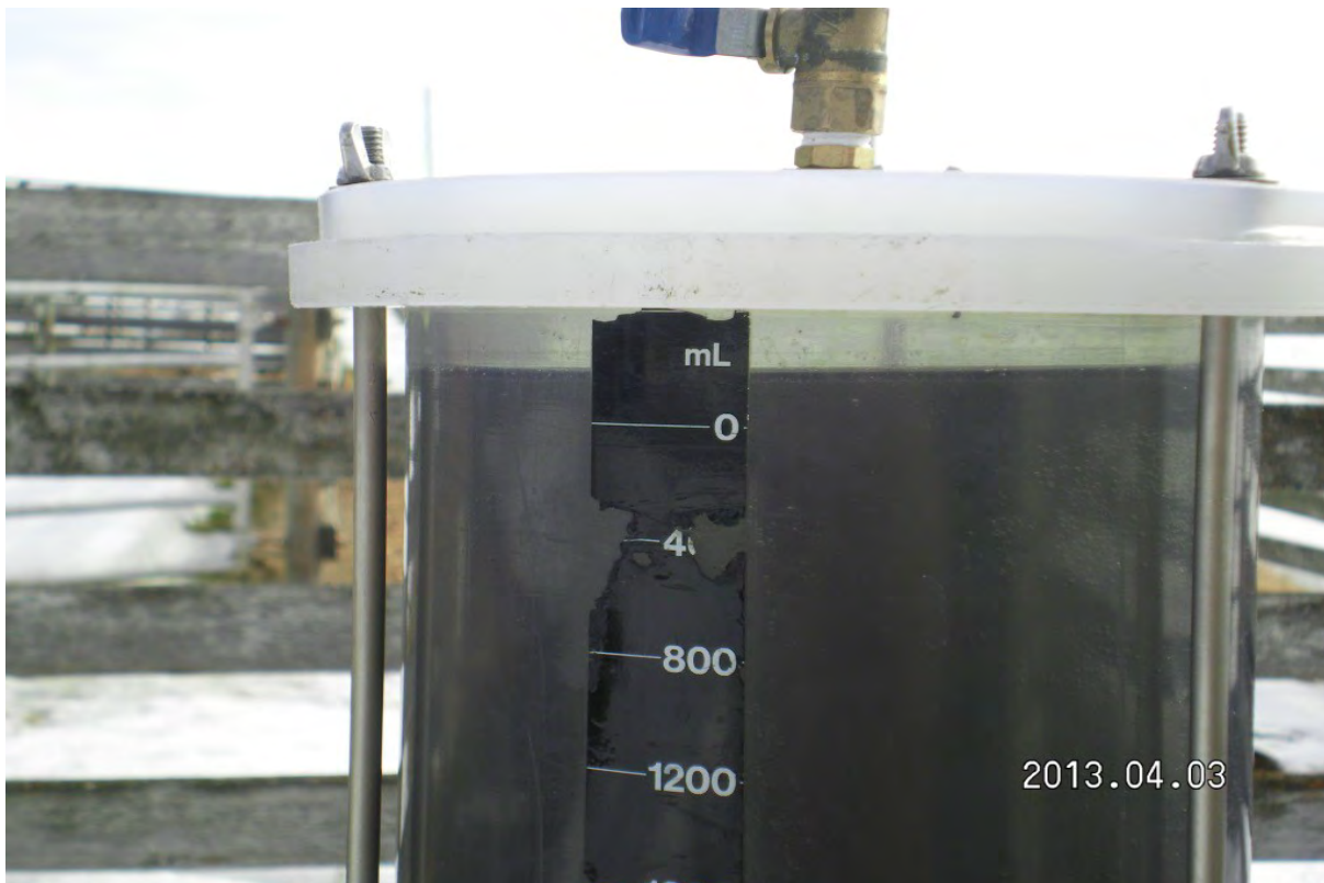
The Campbells' contaminated well water being gas tested in a flow-through cell for the ERCB, April 3, 2013 The black in the cell is the Campbell's water; it took 20 minutes to clear. The well is plastic lined and had not been used for about a year. (Flow-through cells are about 15% efficient. 373 )
