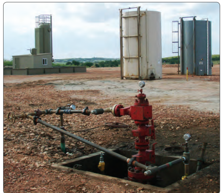
A well head after fracking equipment has been removed from the drilling site.
