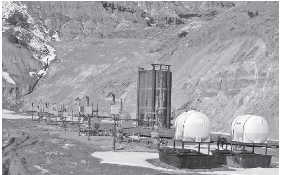
Figure 3: Multiple Wells on a Single Well Pad in Glenwood Springs, Colorado (February 2009)
