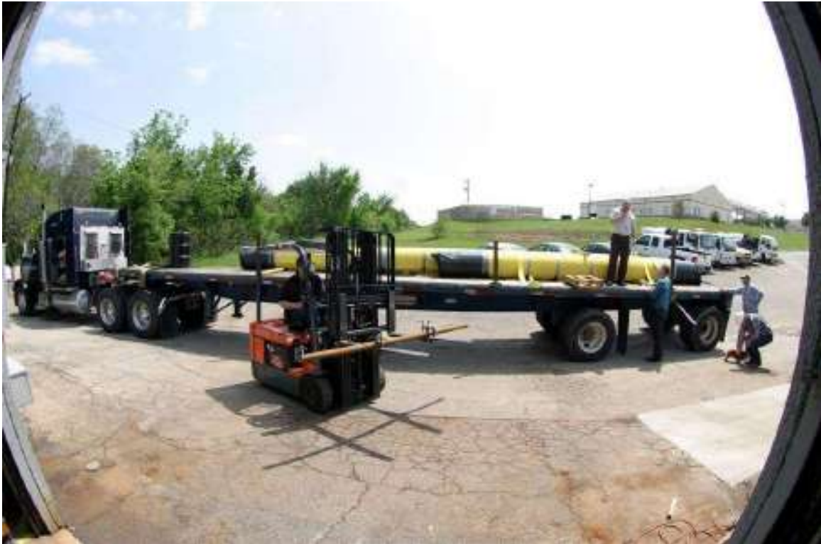
The photograph displays the pipe sections in the as-received condition with the protective wrapping on the outside surface of the pipe sections that was applied to prevent any damage during transportation.
