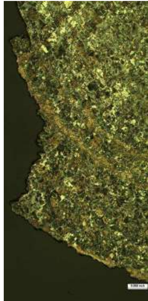
20' 6-13/16" from the North Girth Weld 2% Nital etch, ~100x Photograph No. 182
