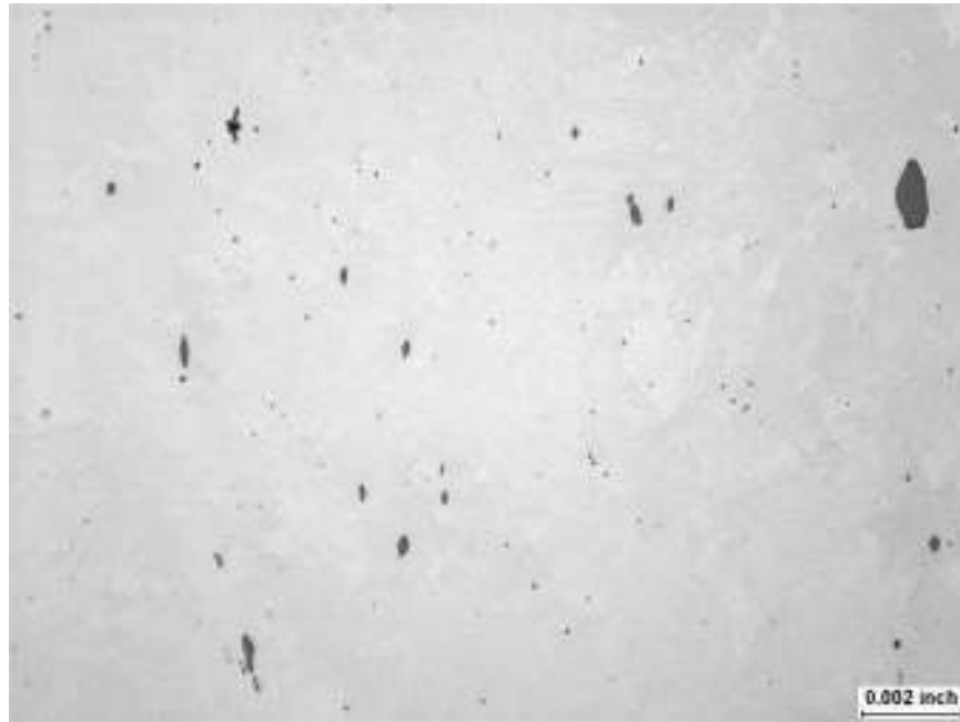
20' 6-13/16" from the North Girth Weld As-polished, ~200x Photograph No. 173
