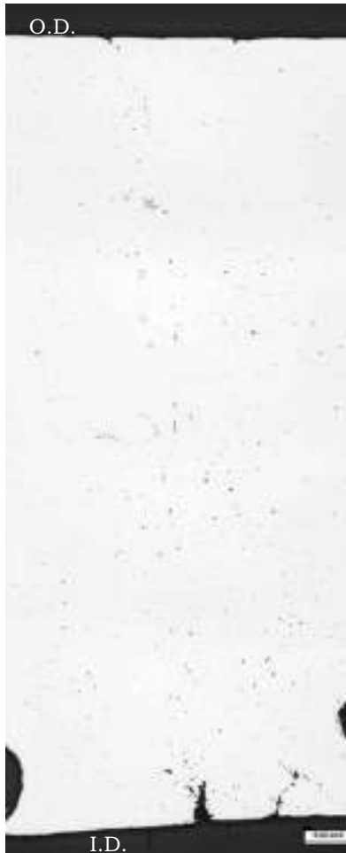
35' 8-1/2" from the North Girth Weld As-polished, ~25x Photograph No. 203
