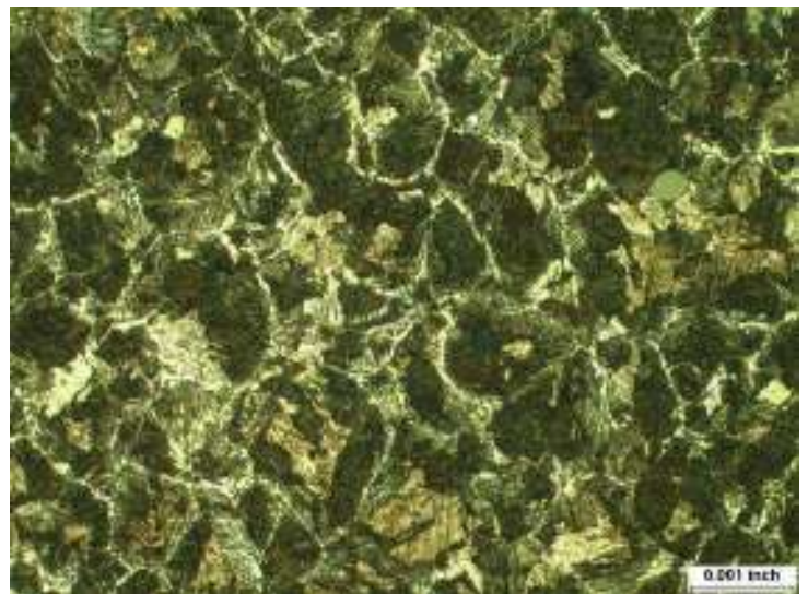
20' 4-7/8" from the North Girth Weld 2% Nital etch, ~500x Photograph No. 169
