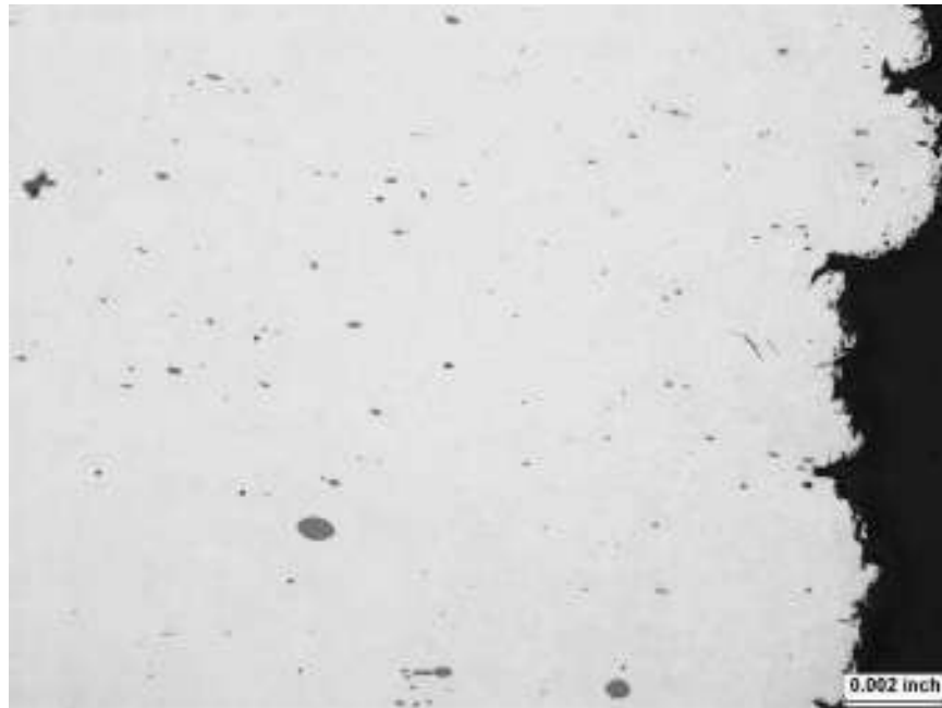
20' 6-13/16" from the North Girth Weld As-polished, ~200x Photograph No. 176
