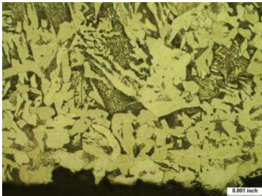
20' 6-13/16" from the North Girth Weld 2% Nital etch, ~500x Photograph No. 188
