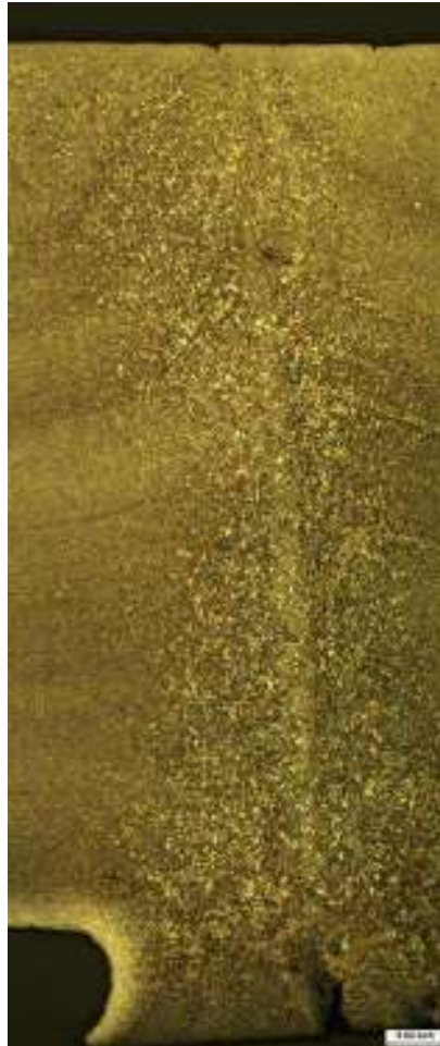
35' 8-1/2" from the North Girth Weld 2% Nital etch, ~25x Photograph No. 215
