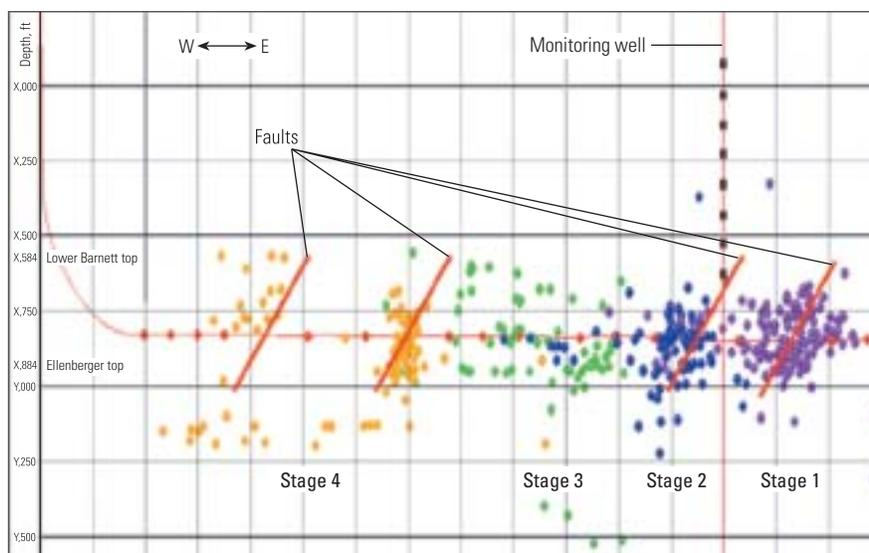
^ Influence of faults on Barnett Shale stimulation. Chesapeake placed perforations along the horizontal completion interval to avoid fracturing into four known faults. Even with the precautions, the StimMAP hydraulic fracture stimulation diagnostics interpretation indicated that the microseismic activity was concentrated around some of the fault planes and influenced by the presence of faults near Stages 1, 2 and 4.
