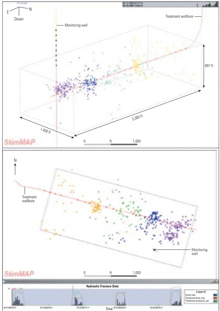
^ Maps of microseismic events from another four-stage hydraulic fracture treatment. The StimMAP displays include a three-dimensional (3D) view (top) and a plan view (middle). The treatment stages are color-coded: Stage 1 is purple, Stage 2 is blue, Stage 3 is green, and Stage 4 is yellow. Also included is a summary of each stage, including acoustically determined fracture system length, width and preferential azimuth (bottom). Depths are given relative to mean sea level (MSL).
