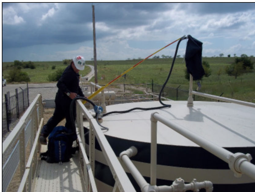
Figure 3.2-3. Sampling a Tank Vent with the Hi Flow Sampler
