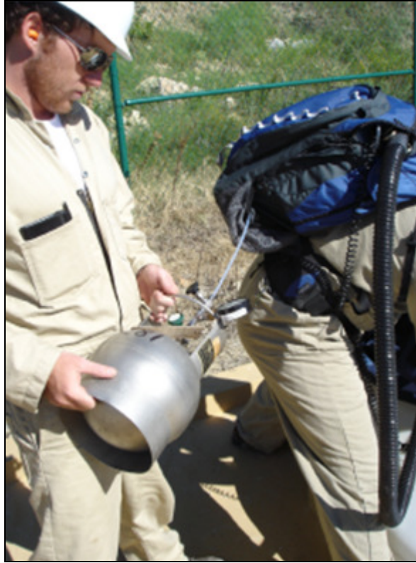
Figure 3.2-4. Collecting a Canister Sample from the Exhaust Port of the Hi Flow Sampler
