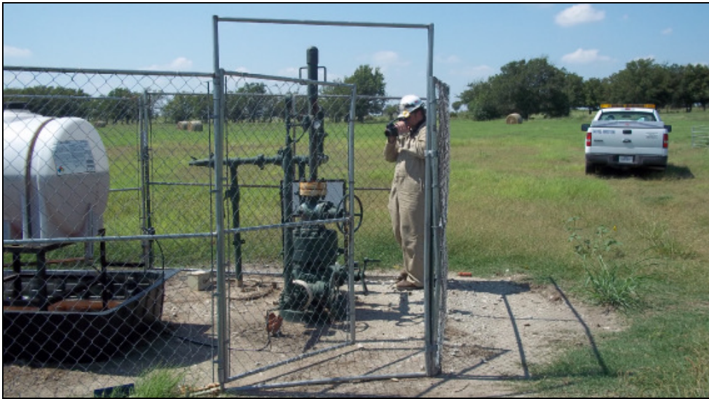
Figure 3.2-1. IR Camera Imaging at a Well Site
