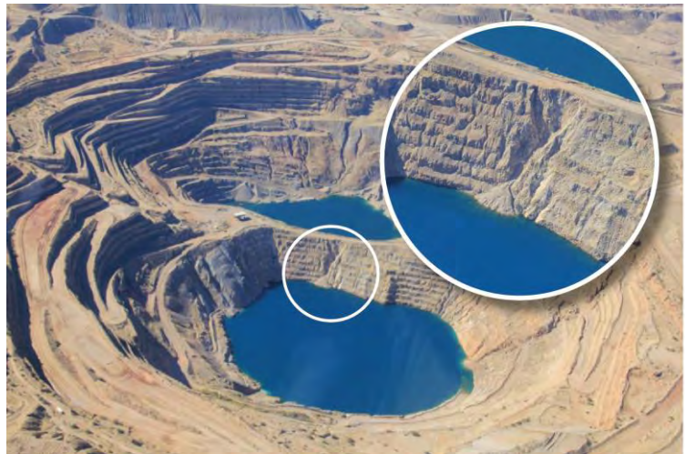
Closed pits and lakes near the Mission Mine Complex, southeast Arizona. For scale, the benches on the right hand photo are probably between 25 and 35 feet high. Photo by Pete Dronkers, Earthworks.
