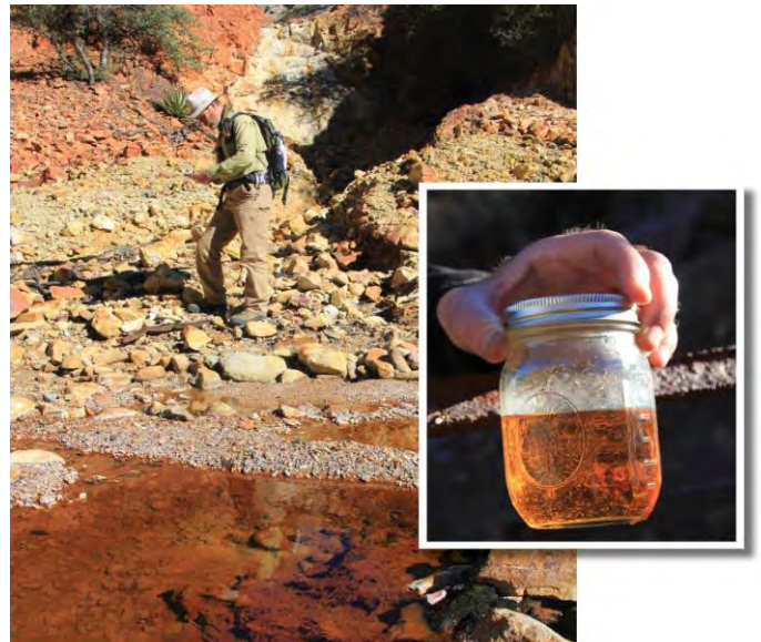
This sample was taken directly from a pool of runoff water at a small abandoned mine in the Patagonia Mountains, a few miles away from the proposed Hermosa Mine. The water was later tested for acidity, and checked in at pH 2.5 – comparable to vinegar or lemon juice, and about five orders of magnitude more acidic than distilled water. The Hermosa mine would be many thousands of times larger than this mine and could generate proportional volumes of acidic water. Photo by Pete Dronkers, Earthworks.
