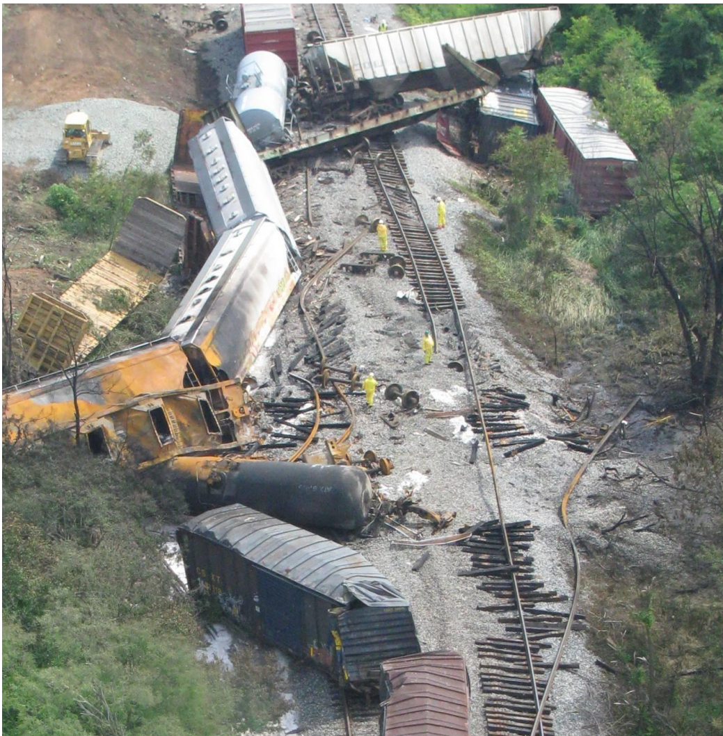
Figure 5. Aerial photograph, May 29, 2013, showing explosion site, derailed cars, and damaged tracks.
