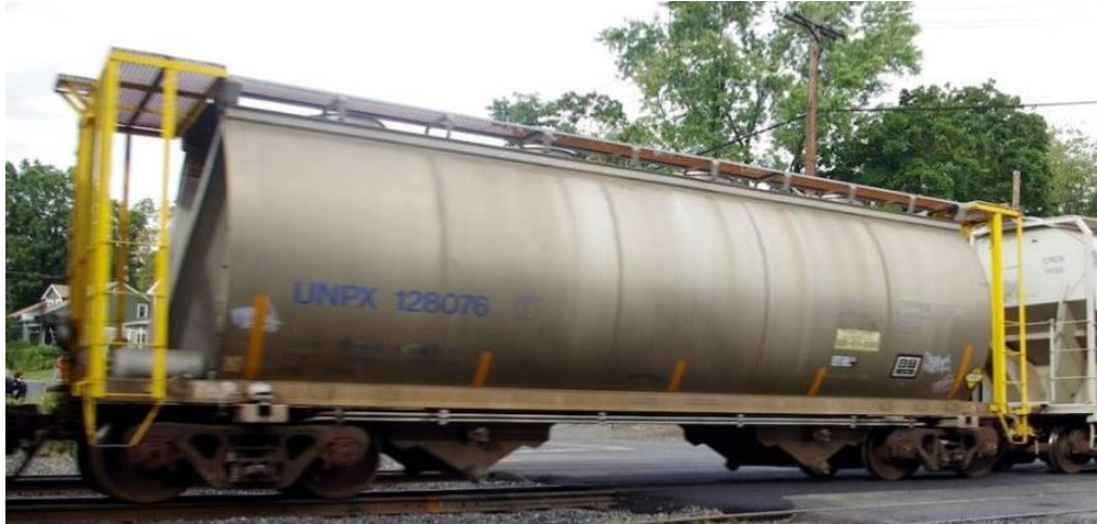
Figure 12. Precrash photo of cylindrical aluminum covered sodium chlorate hopper car UNPX 128076, September 29, 2012. (Source: Railroad Picture Archives)
