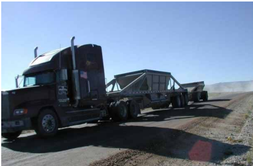
Dust Control — Examples and Illustrations. Treated and untreated sections of road. Dust Suppressant — good reduction in dust. (Dust trail still visible where there was no treatment.)
