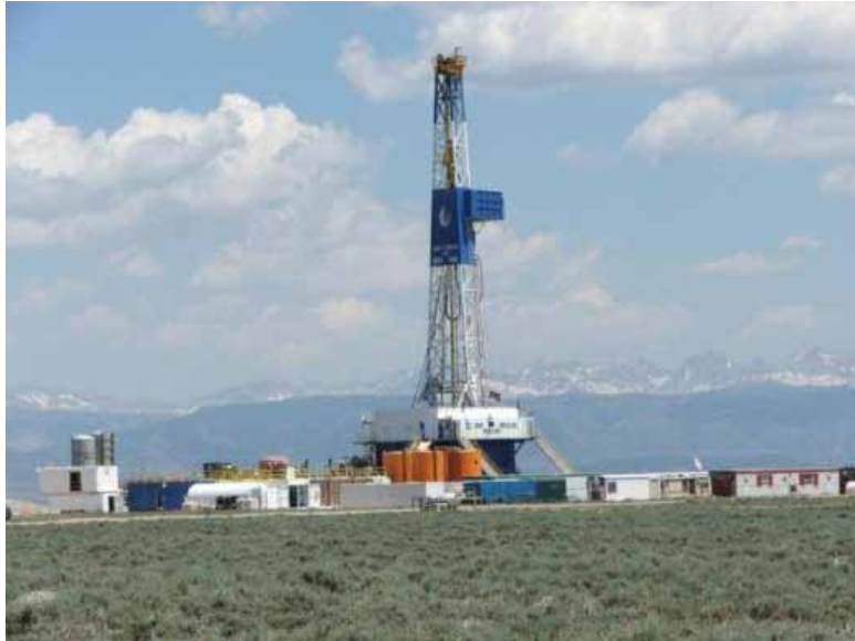
A Tier 2 diesel engine powers an electric motor to drill this well.
